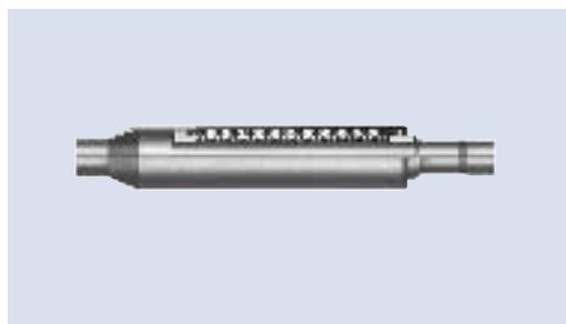
Bellows made of bronze, soldering ends on both sides made of copper with external sleeve made of copper, prestressed
