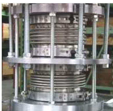
Movement test to determine the stress cycles endured.
