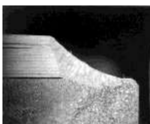
Macro cross section of an inner welding seam
