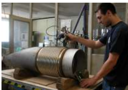
Helium leak test
