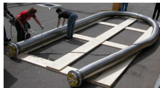
Oxygen lance for steel plant, DUO® DN250/PN16, length 18 m, produced in one piece
