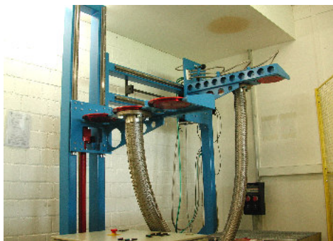
U-bend test to determinate the achievable number of cycles
